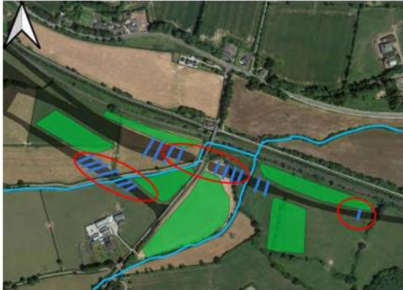
Figure 5-376 Indicative location of flood relief culverts (in red)
